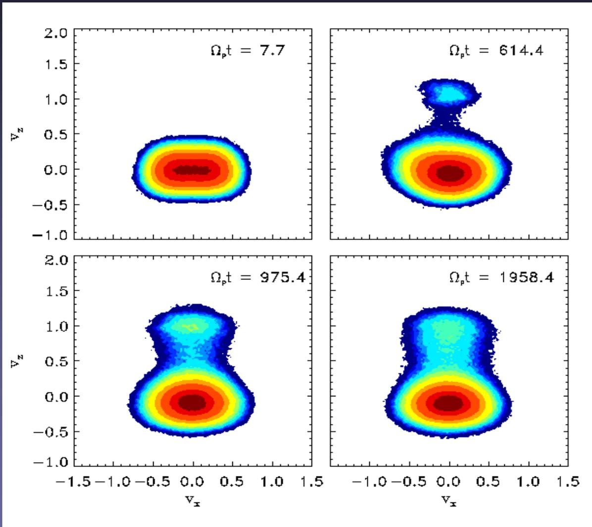
VDFs as obtained by numerical simulation of the decay of Alfvén-cyclotron waves and the related ion kinetics
