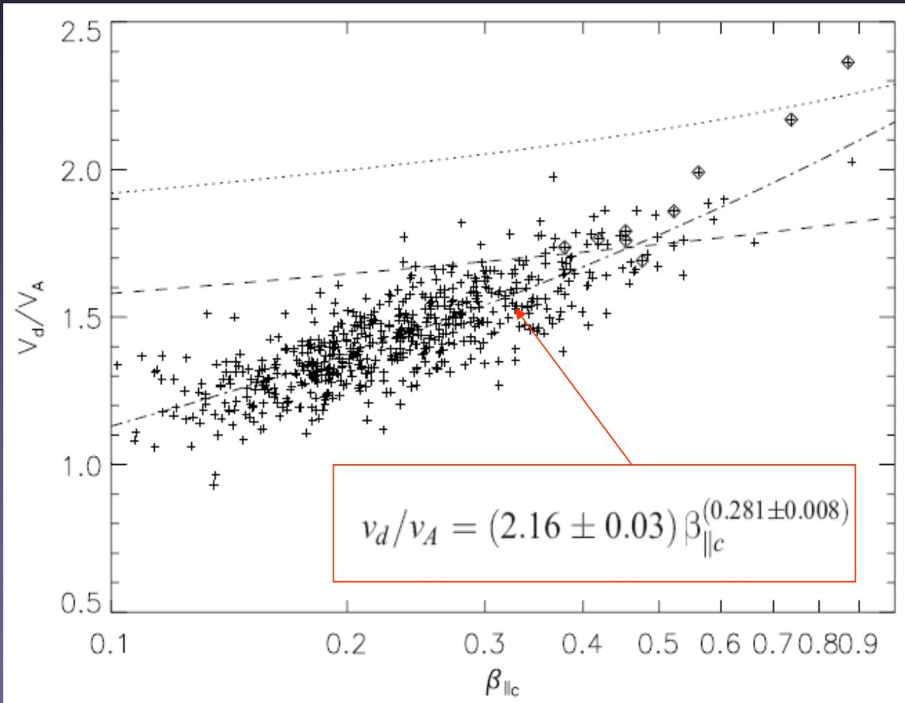
The dotted and the dashed lines show the threshold of the Alfvén I instability (Daughton and Gary, 1998) with a constant ratio of the proton beam density to the electron density, for the values 0.05 (top) and 0.2 (bottom line).
