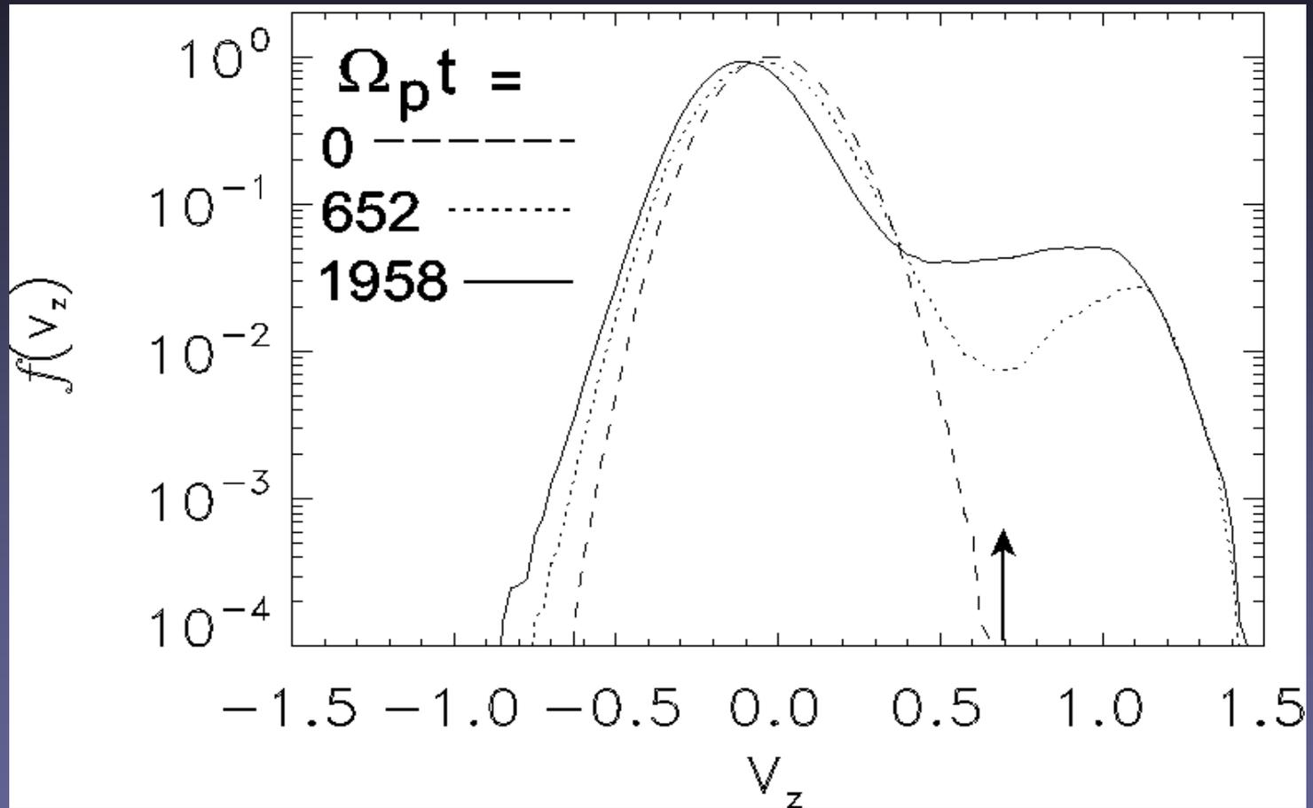
**Numerical simulation results:** One-dimensional cuts through the proton VDF as a function of  $v_z$  along the magnetic field direction for the dispersive-wave case at three instants of time. Note the formation of a beam with a final relative density of about 7%.
